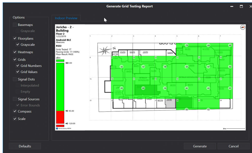
Figure 8: Formal grid report showing floor plan with heat map overlay
