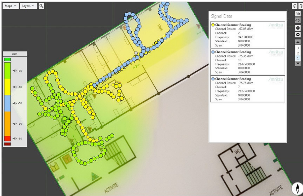
Figure 9: Results of a multi-frequency coverage mapping measurement in NEON Command software
