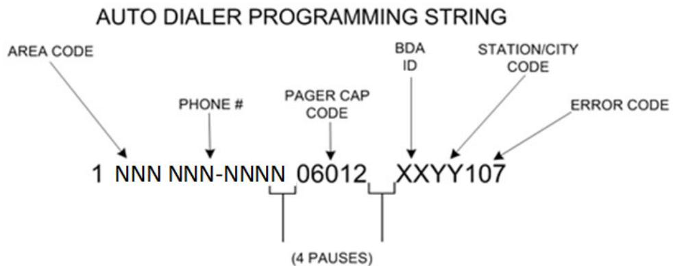
The OCSD/COMM 900 MHz Paging System phone number will be provided during plans review. You will need to program pauses (usually 4 each) between the number dialed, cap code and BDA ID for the auto dialer to function properly into the County's 900MHz paging system.
